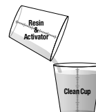
Pour mixed Resin & Activator into new clean container Mix thoroughly for an additional 3 minutes.
