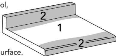
2. Next, use the Sanding Block to sand the backsplash and front edge. Since the Sanding Block has fully textured sides, it is used to get into tight spots the curved backsplash and front edge. You only need enough pressure to create a smooth, lightly textured surface. Do not sand through the chips.
